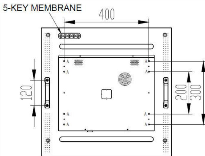
A : 8-M6\_USER HOLE\_MAX. DEPTH=20mm
